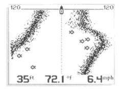
When a Wide Side transducer is connected, the screen display changes to display the information from the side-locking elements. There are four basic views available when the Wide Side transducer is in use; both, left, right, and down. These views are controlled by the VIEW button. The default view is both, in which information from both the left and right elements are displayed on-screen. The digital depth of the water beneath your boat is always present.
